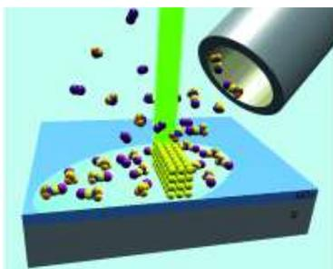
Figure 2 Schematic of EBID
