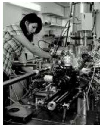
Figure 1 Low temperature STM at Bath
