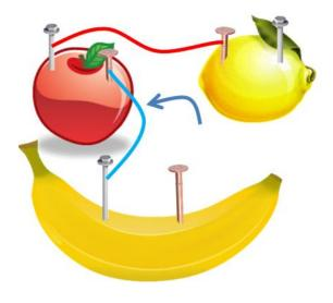
3. Make sure to connect the copper nail to the long part of the LED.
