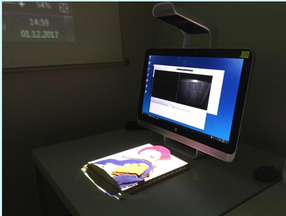
The sprout colours the different sections of a reliefs and identifies the hand movement.
